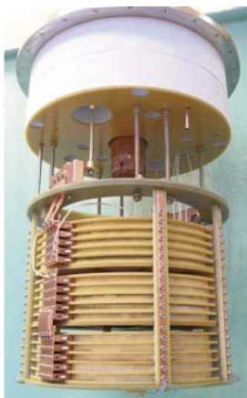
2.2 MVA FCL demonstrator tested within the joint AMSC/Siemens development agreement
